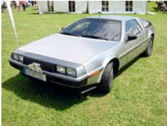
The **DeLorean DMC-12** (commonly referred to simply as **The DeLorean** as it was the only model ever produced by the company) is a sports car manufactured by John DoLorean's DoLorean Motor Company for the American market in 1981-82. Featuring gull-wing doors with a fiberglass "underbody", to which non-structural brushed stainless steel panels are affixed, the car
